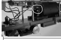
Oil both ends of motor shaft where it passes thru the motor bearing. The flywheel end requires a thin tube oiler to get between the flywheel and the motor housing.
