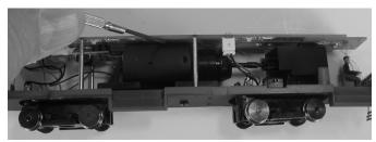
3. Gently pry circuit board off the mounting posts.
