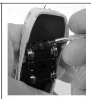
2. Start with the rear end. With body spread from step 1, slide a small screwdriver into the truck opening and pull the mechanism out a little. Repeat step 1 and 2 for front end.
